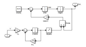
The Magnetic Ball Plant model represents an iron ball of mass M. This ball moves under the influence of the gravitational force, Mg, and an induced
